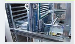
The extractor delivers the requested tray to the access opening or returns a tray to a location within the unit at fast speeds. Both vertical and horizontal travel speeds can be adjusted to accommodate sensitive items.
