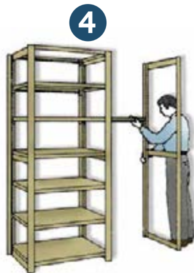
4 ADD EXTRA SECTIONS Utilize common center Uprights. (An additional Upright must be used to add extra sections.)
