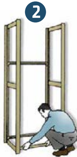
2 BUILD FROM THE BOTTOM UP Place Shelf Supports or Quik-Base (front and back) for lowest shelf only.
