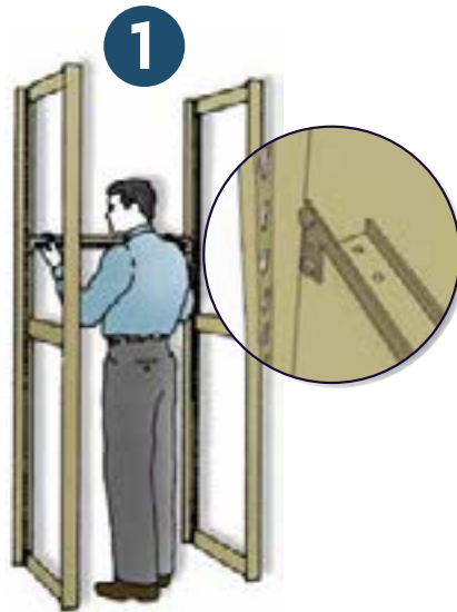
1 POSITION UPRIGHT Temporarily place one Shelf Support at any convenient location to properly space Uprights.
